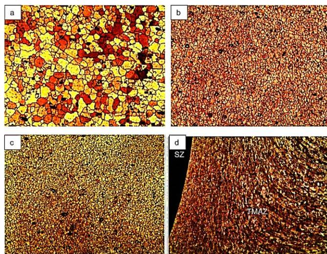
Figure 2: Microscopic images showing grain sizes of: (a) base material; (b) after FSP without RPs; (c) after FSP with CNTs as RPs; and (d) interface of composite with upward flow pattern [38].
