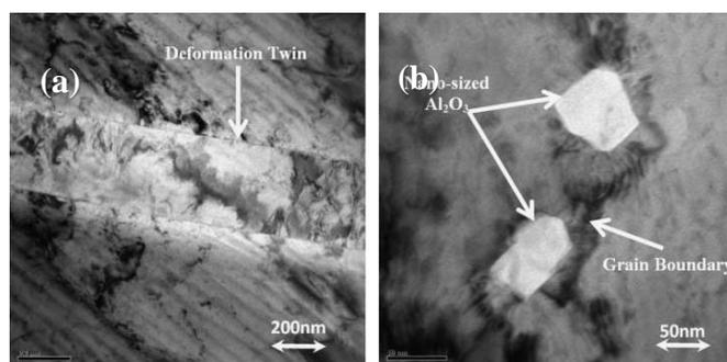
Figure 3: TEM microstructure of Ti/Al<sub>2</sub>O<sub>3</sub>, (a) deformation twin in the Ti-20n-0.8 sample, (b) pinning of grain boundary by two nanoparticles [39].
